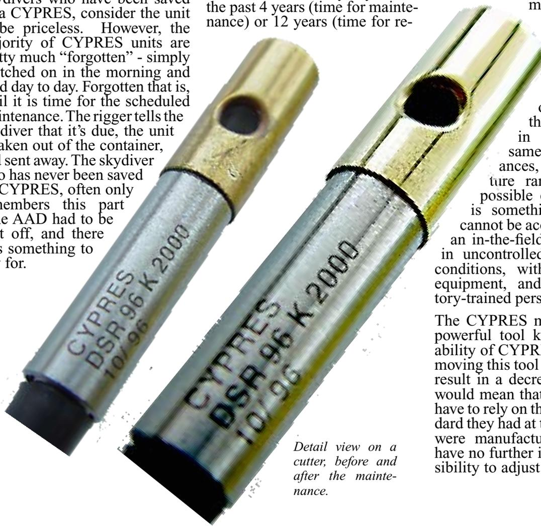
*Detail view on a cutter, before and after the maintenance.*
