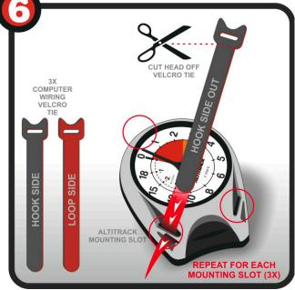
Slip a Velcro wire tie through each of the mounting slots on the Altitrack. Make sure the hook side is facing OUT. Snip off the heads of the wire ties.
