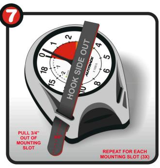
7. Pull each velcro tab through the mounting slot 3/4"
