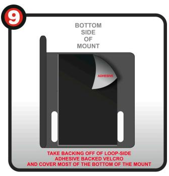
Peel the backing of of the large loop-side piece of velcro with the adhesive backing and adhere it to the bottom underside of the altimeter mount.
