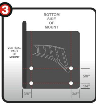
3. Using the 1/8" drill bit and drill, drill holes where the dimension lines cross.
