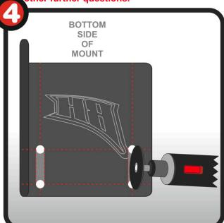
4. Use a Dremel or Rotary tool to remove the material in between the holes. Be careful and go slow.
