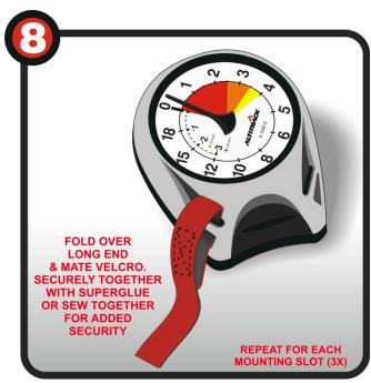
8. Fold the long end of the velcro tab over and mate it to the short end. You can use either super glue or sew the loop together. Do this for each of the 3 tabs.
