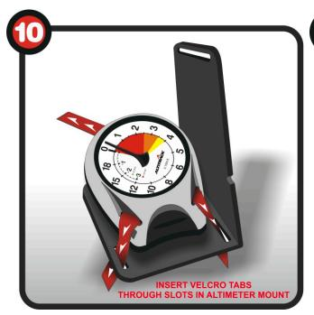
10. Slip the 2 rear tabs through the slots you cut in the altimeter mount.
