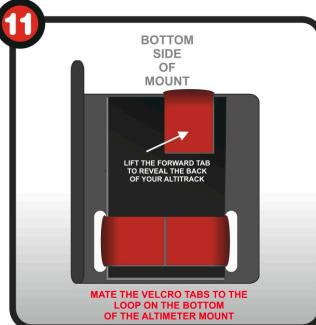
11. Mate the velcro tabs to the loop velcro on the bottom of the altimeter mount. The single forward tab can be released to flip the altimeter over to use the computer functions.
