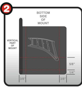
2. Measure out the above dimensional grid to determine slot and drilling placements.
