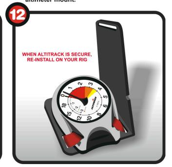
12. Re-install on your rig following manufacturer's reccomended instructions. Check your mount during each pack job to ensure your Altitrack is secure and ready to jump.
