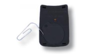
Press a paperclip into the tiny hole on the rear side of the unit and release. The unit restarts.
