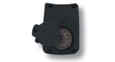
Carefully remove screw from battery cover and remove batteries. Install new batteries and note polarity. Use only Renata CR-2325
